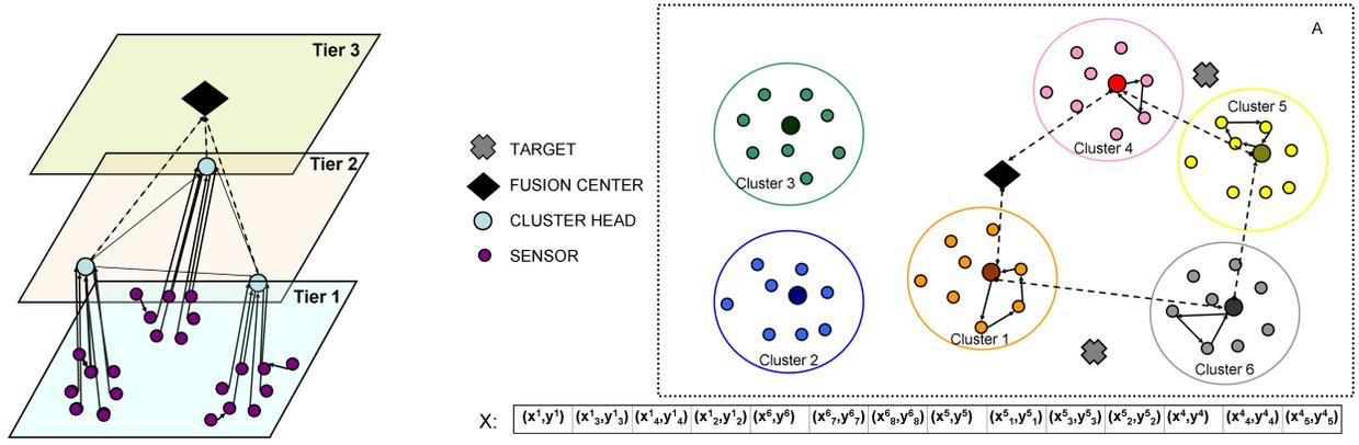
Fig. 1. A hierarchical WSN (left) and an example of a mobile agent route with its encoding representation (right)
