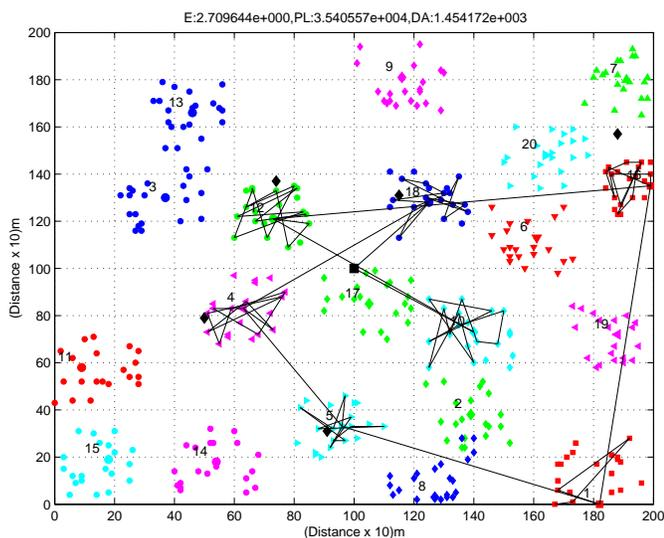
Fig. 6. The mobile agent route obtained by EMOCA that provides the highest data accuracy for test instance T8.
