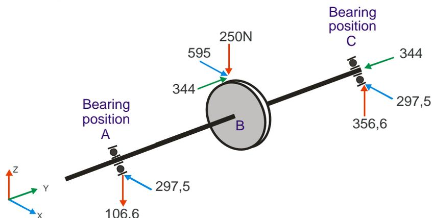
Fig. 1: Shaft supported with bearings
