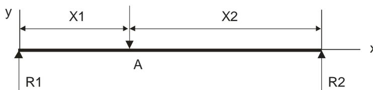
**Figure:** Simply supported shaft
