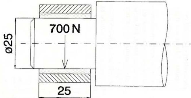
**Fig. 2.7** Boundary lubricated bearing design example.
